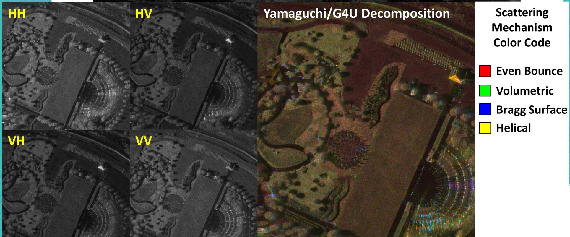
SNL FARAD, X Band, 0.2m Full-Pol Imagery of New Mexico Veterans Memorial, Model Based Decomposition Example
