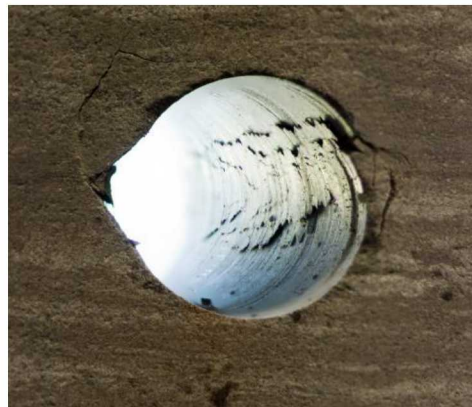
Borehole breakout in Mancos Shale
