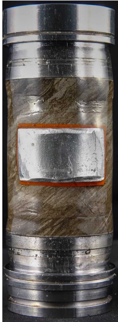
Prepped Mancos Shale sample
