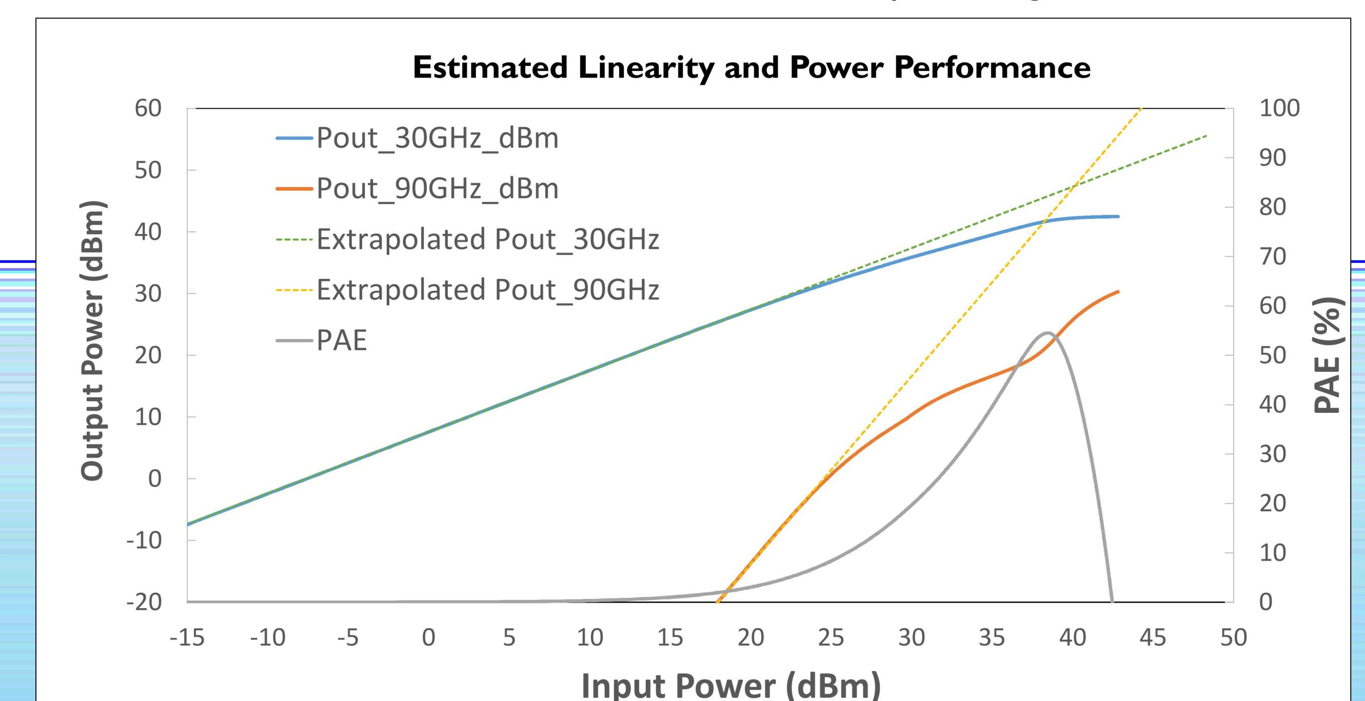
Simulation results indicate that a saturated power density of 18 W/mm with 55% PAE and OIP3 of over 40 dBm can be achieved for this device.
