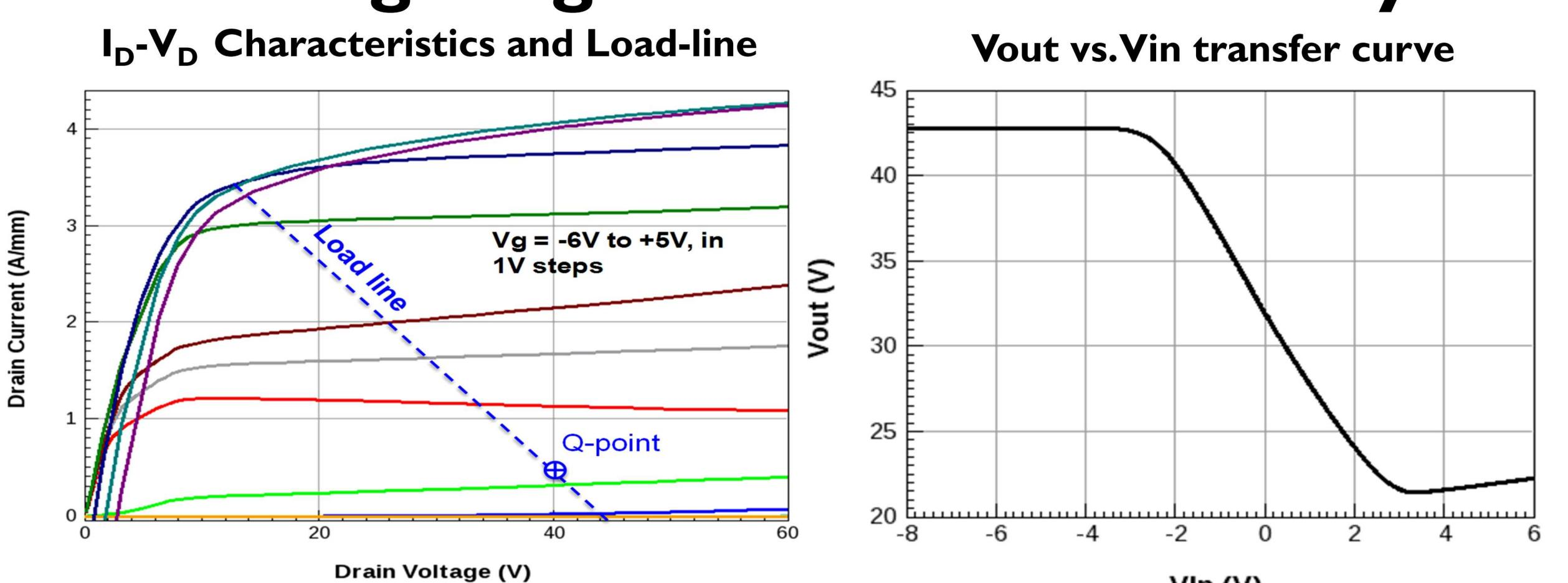
The  $V_{out}$  vs.  $V_{in}$  transfer curve was obtained from DC sweep simulations using a resistive load-line and a Q-point selected for maximum output voltage swing.
