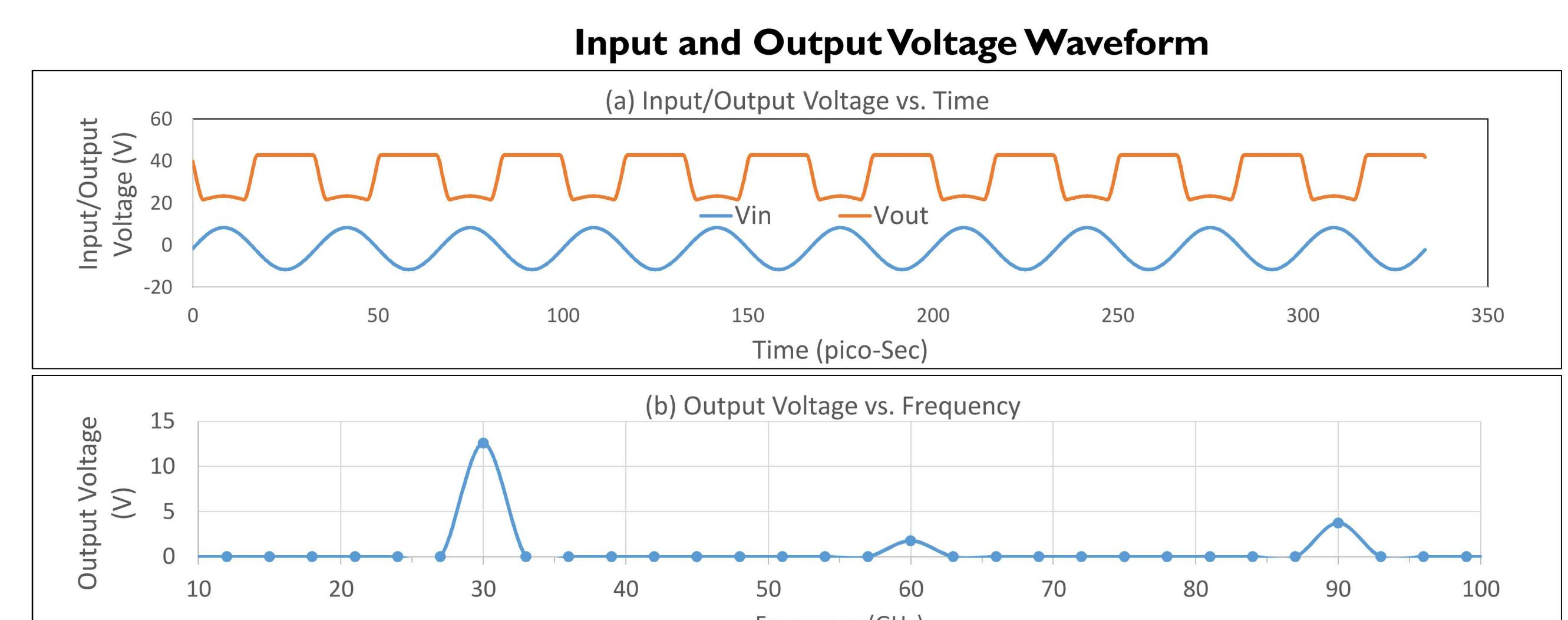
A MATLAB-based algorithm was used to calculate the output power waveforms for a sinusoidal 30 GHz input. The output powers 3rd harmonic performance, and PAE were calculated from the Fourier transform of the output voltage waveform.
