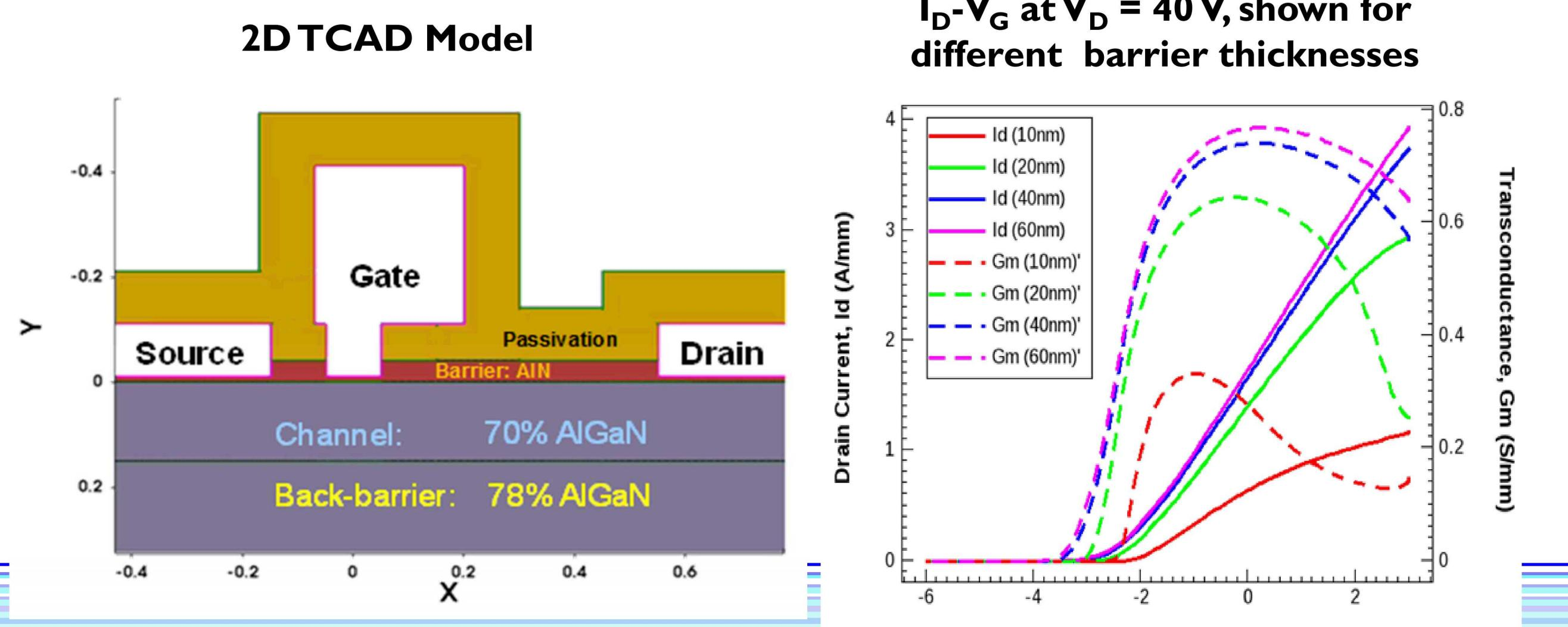
Physics-based TCAD model for Al-rich AlGaN channel HEMT, created in the Sentaurus® simulation platform, was used for device simulation. A design of experiments based on small-signal TCAD simulation results was used for device optimization.
