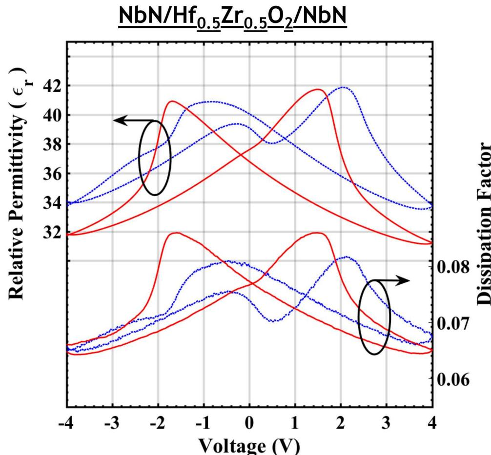
Relative permittivity and dissipation factor at 100 kHz as voltage is swept from -4 V to 4 V and then from 4 V to -4 V at room temperature before (blue dot) and after a 360 second, +/- 4 V and 1 Hz wakeup at room temperature (red line).
