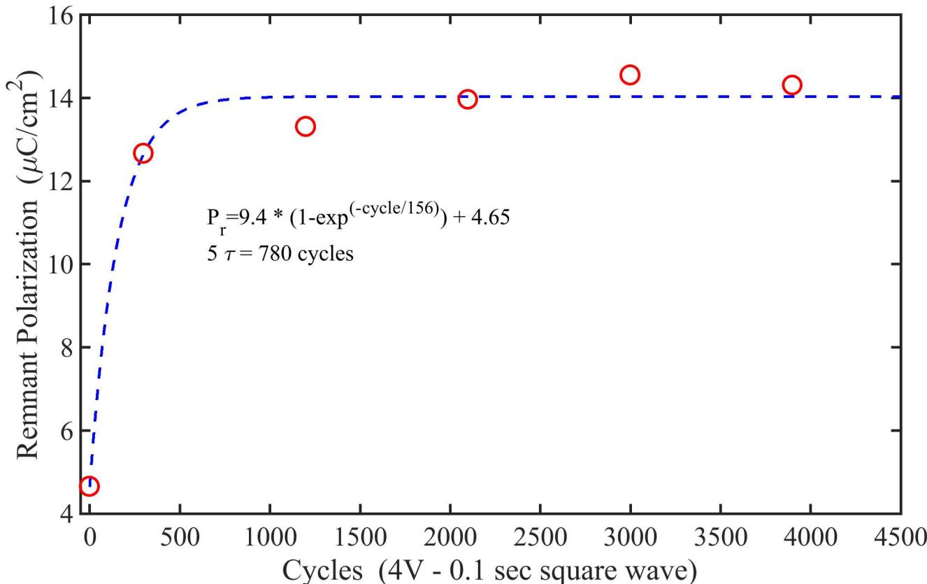
Wake up in a 77  $\mu\text{m}$  radius NbN/HfZrO<sub>2</sub>/NbN ferroelectric capacitor with a 20 nm film thickness using a 4 volt, 10 Hz cycle.
