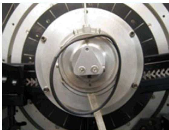
Figure 4. Failure seen with Viton O-ring due to sCO 2 exposure
