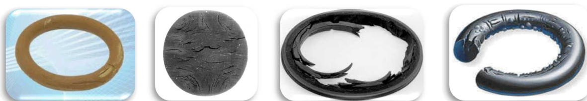
Figure 3. Examples of failures in elastomers in sCO 2 service due to explosive decompression
