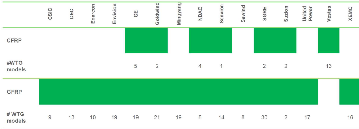
Figure 1-5. Breakdown of turbine models with carbon fiber spar caps for the top 15 OEMs.
