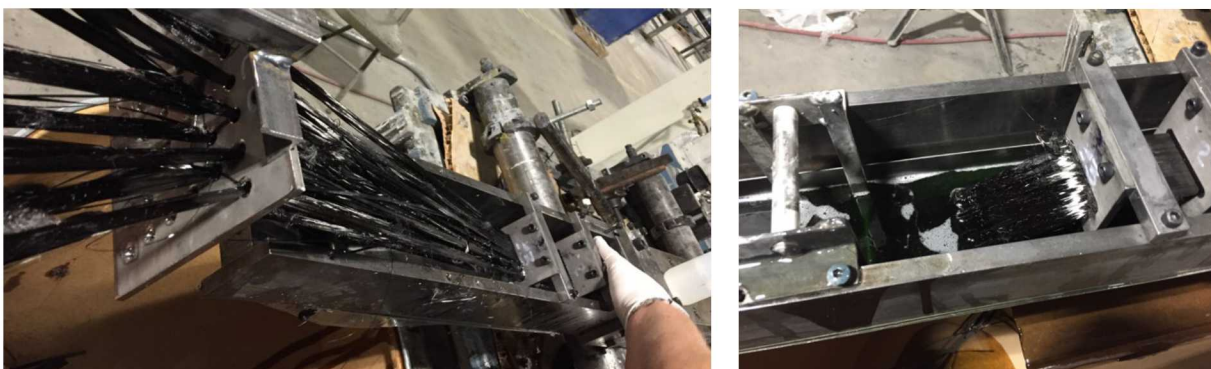
Figure 2-9. CFTF material being dipped through resin and pulled through the pultrusion die.
