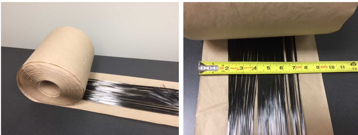
Figure 2-6. Example of initial heavy-tow CFTF material winding.
