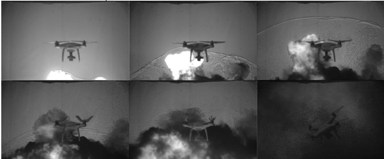
Figure 2-2. Shock wave hits the UAV from below, bending the propellers and destabilizing the UAV.
