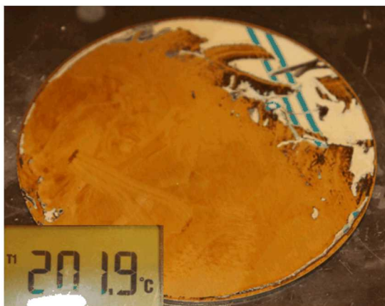
Figure A-2. Picture of steel sample after heating to 200 °C (392 °F) showing the blackened adhesive residue left on the surface).
