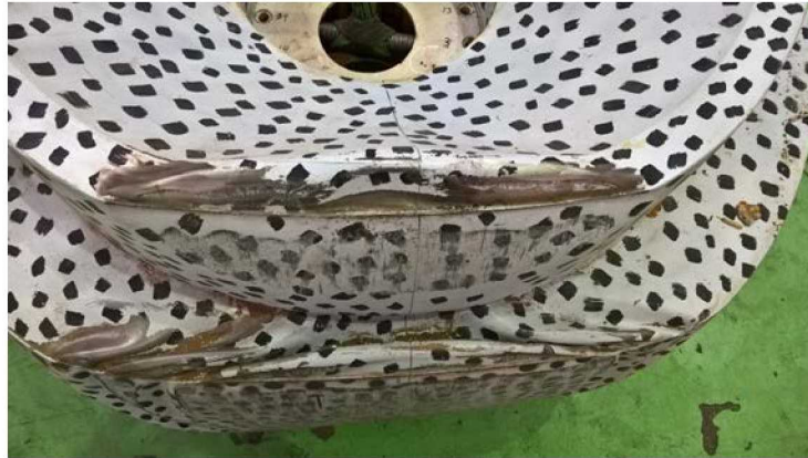
Figure 2-6. Damaged Bottom Impact Limiter.
