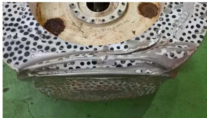
Figure 2-5. Damaged Bottom Impact Limiter that was Modified for Use as a Top Impact Limiter.
