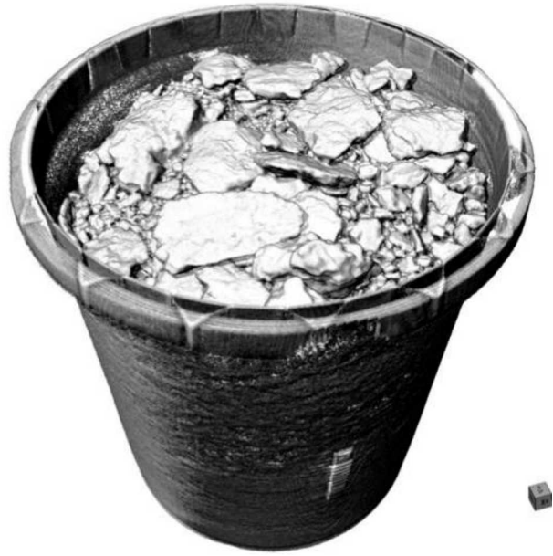
Figure 7-2. X-ray tomographic reconstruction of bucket of run-of-mine salt. The bucket is approximately 12" across.
