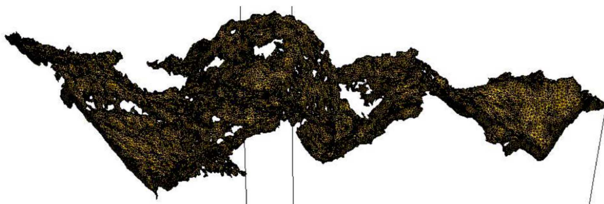
Figure 7-13. Triangular CFD mesh of WIPP DRZ core piece fracture.
