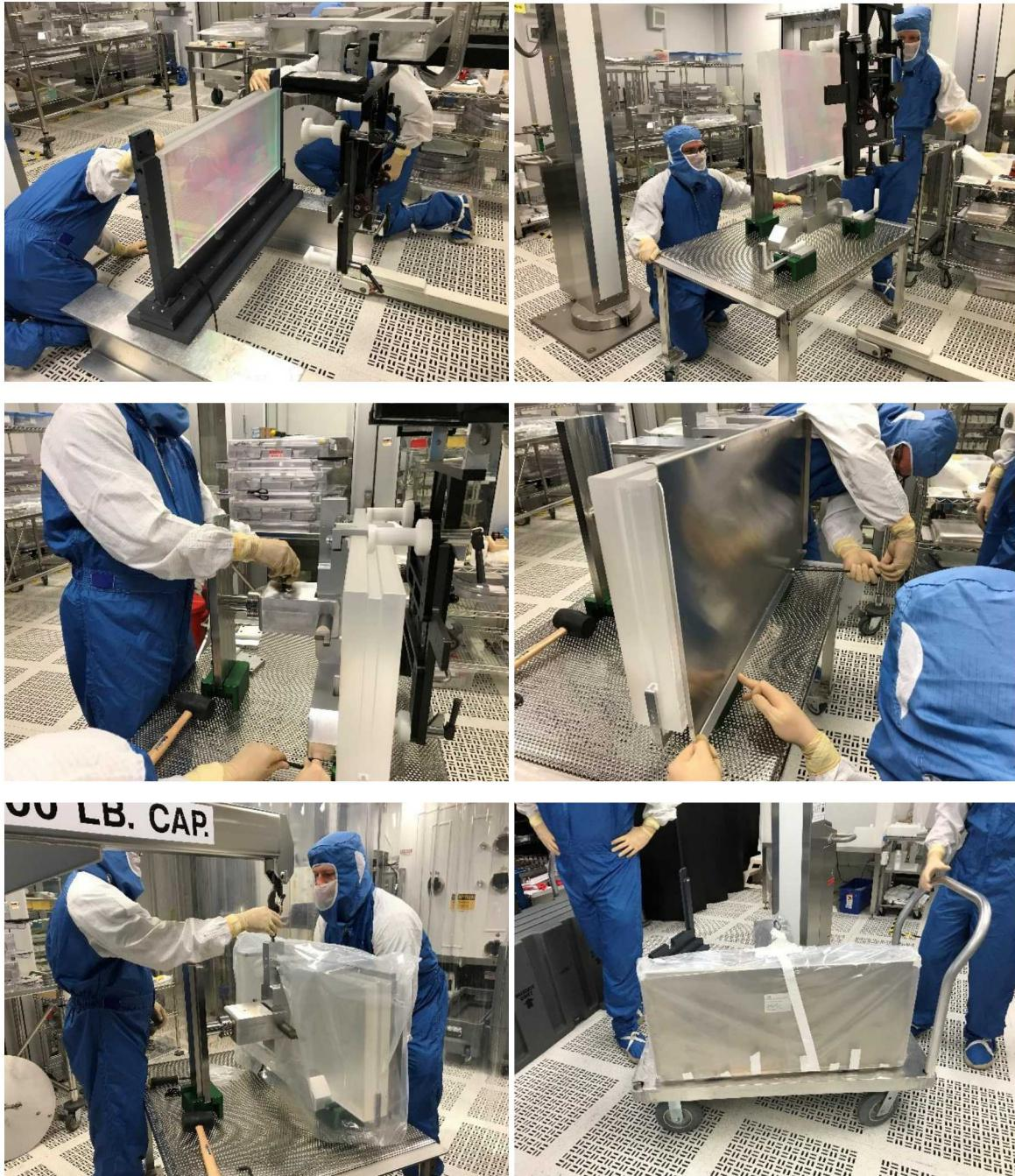
Dichroic beam combiner for co-injection (one of two):
