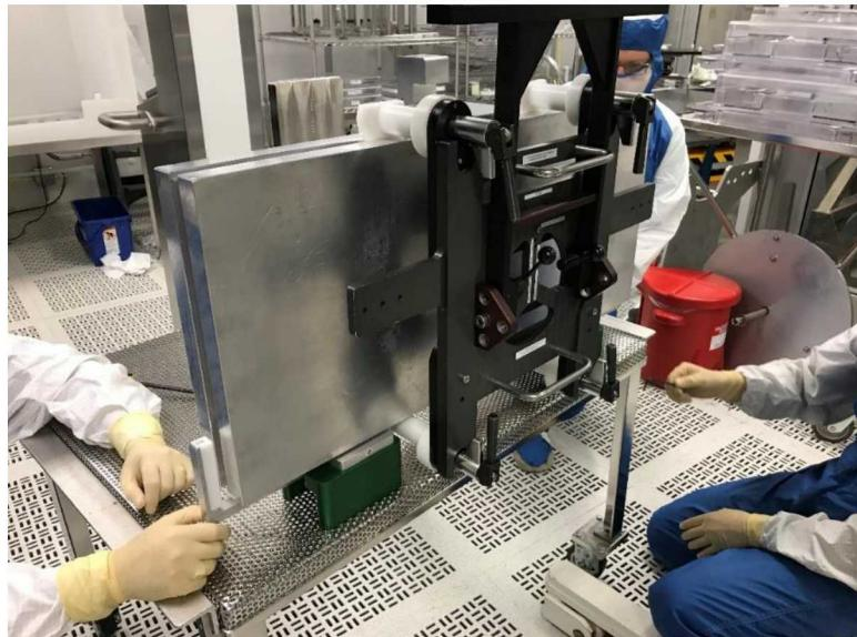
Installation of one of four of the large gratings into custom mount:
