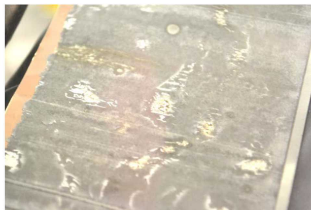
Figure 2: Cell teardown picture of standard graphite anode with clear evidence of plated lithium.
