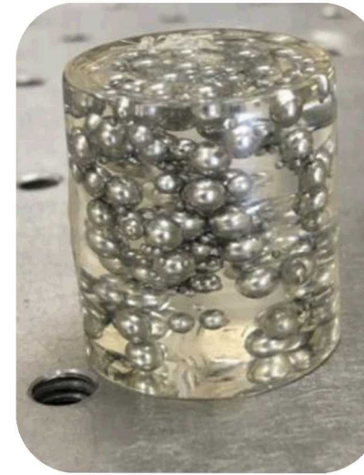
Epoxy seeded with aluminum spheres
