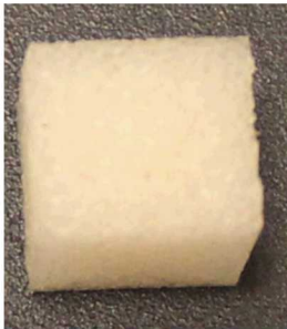
Cellular Silicone 37 pcf (592 kg/m 3 ) Porosity: 47%
