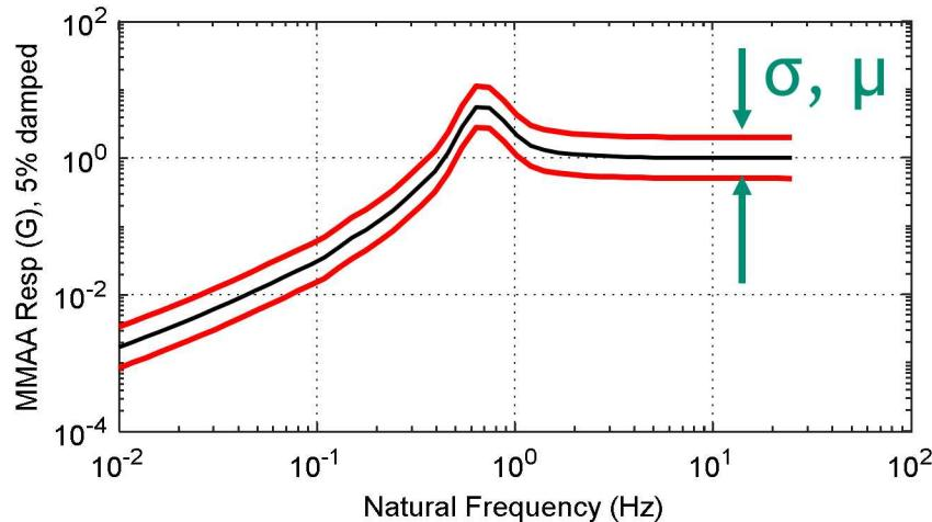
The shock response spectrum is ill-equipped to describe transient motion.
