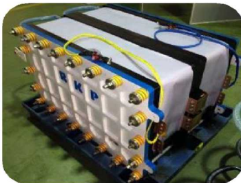
32 KW Stack Rongke Power/UT 120 mA/cm 2 Meter size stack
