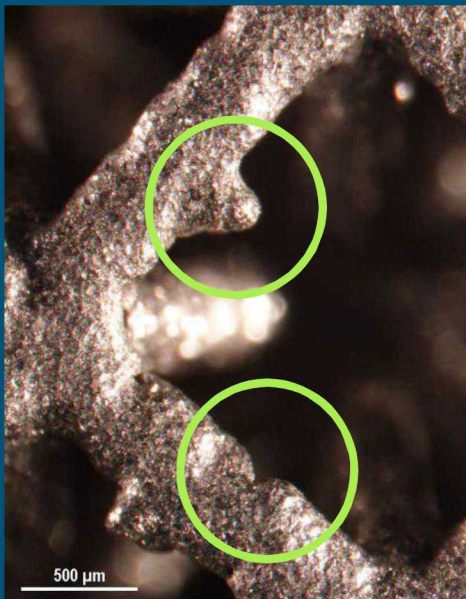
Extra and missing material
