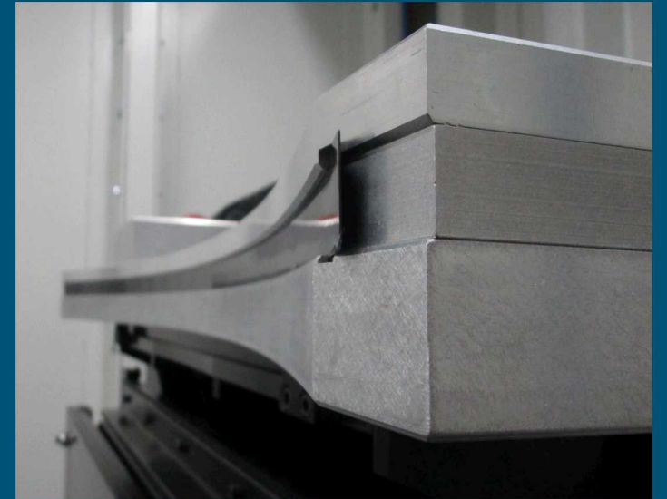
CLDA contains a single row of pixels, reducing scatter and improving signal to noise ratio
