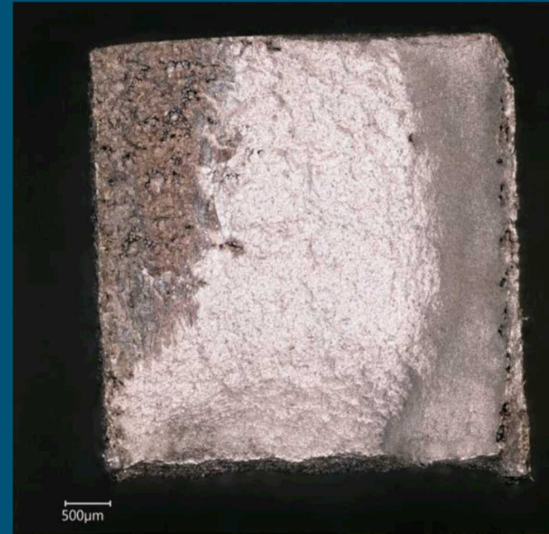
Surface of fracture site
