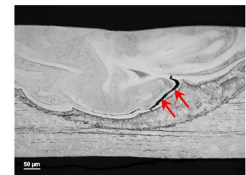
Solidification defect in dissimilar Ni/304LSS laser spot weld
