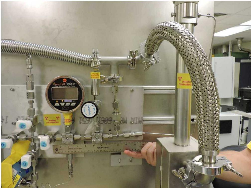
Currently used for tritium gas mixes- internal tritium contamination exists at low levels
