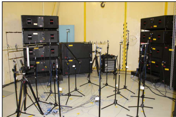
Large Reverberation Chamber (20' x 25' x 30')
