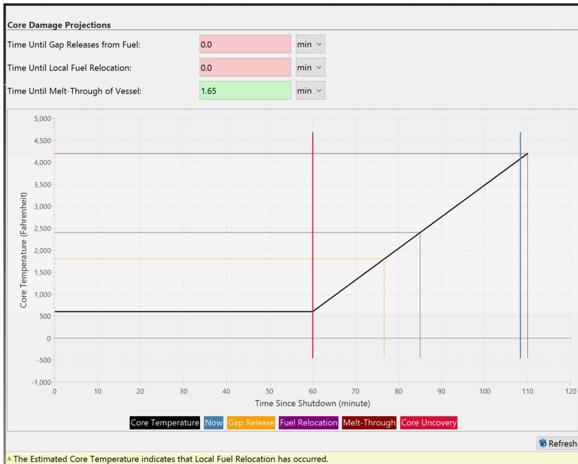
Figure 6. Core Damage Projections Provided by the RTT, based upon the time of core uncovery.
