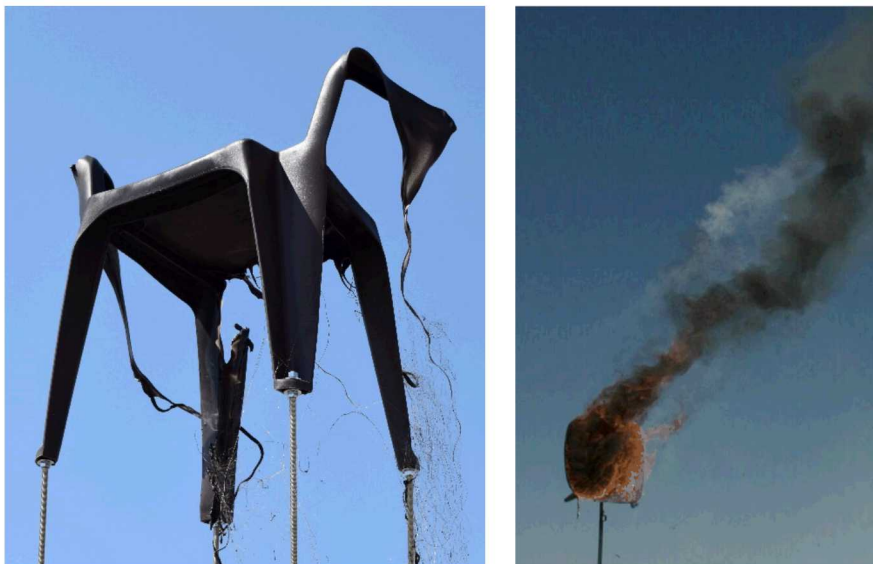
Fig. 7. Post-exposure flaming of the polypropylene chair (left) and the fabric chair (right)
