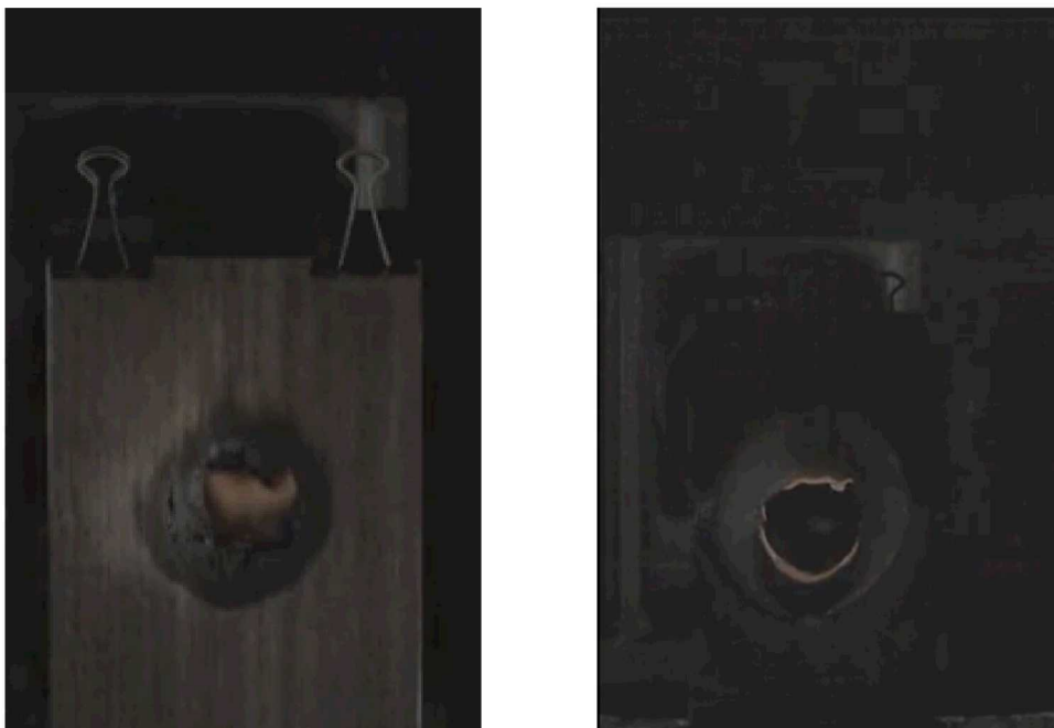
Fig. 3. Two thin rectangular Solar Furnace samples exhibiting sustained flaming at/within the rim of the hole. The left figure is a walnut veneer at 3.5 seconds, and the right figure is black polystyrene at 3.5 seconds.
