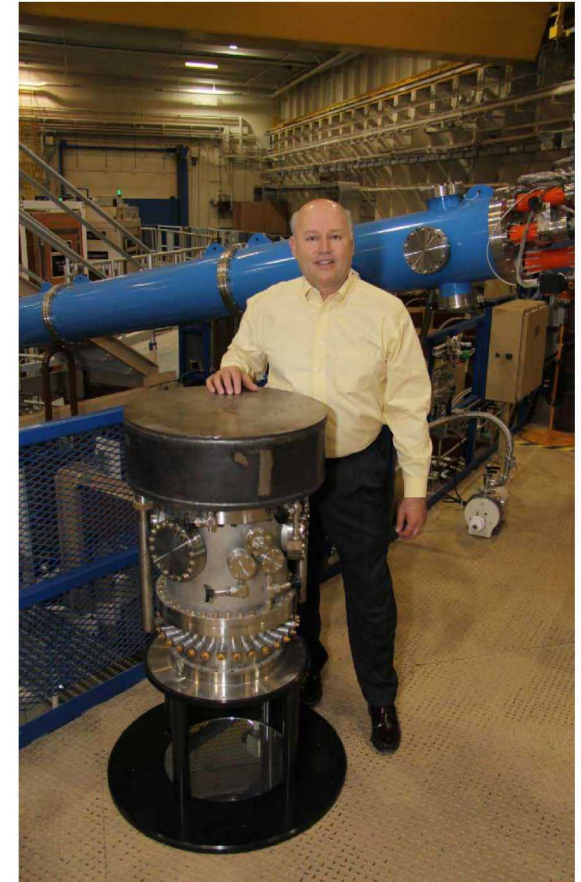
Image of Z explosive containment system used to contain debris from experiments with hazardous materials such as plutonium
