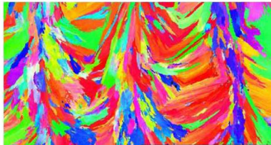
Image from electron backscattering diagnostic of grains in an additively-manufactured stainless steel. The different colors represent different grain orientations.
