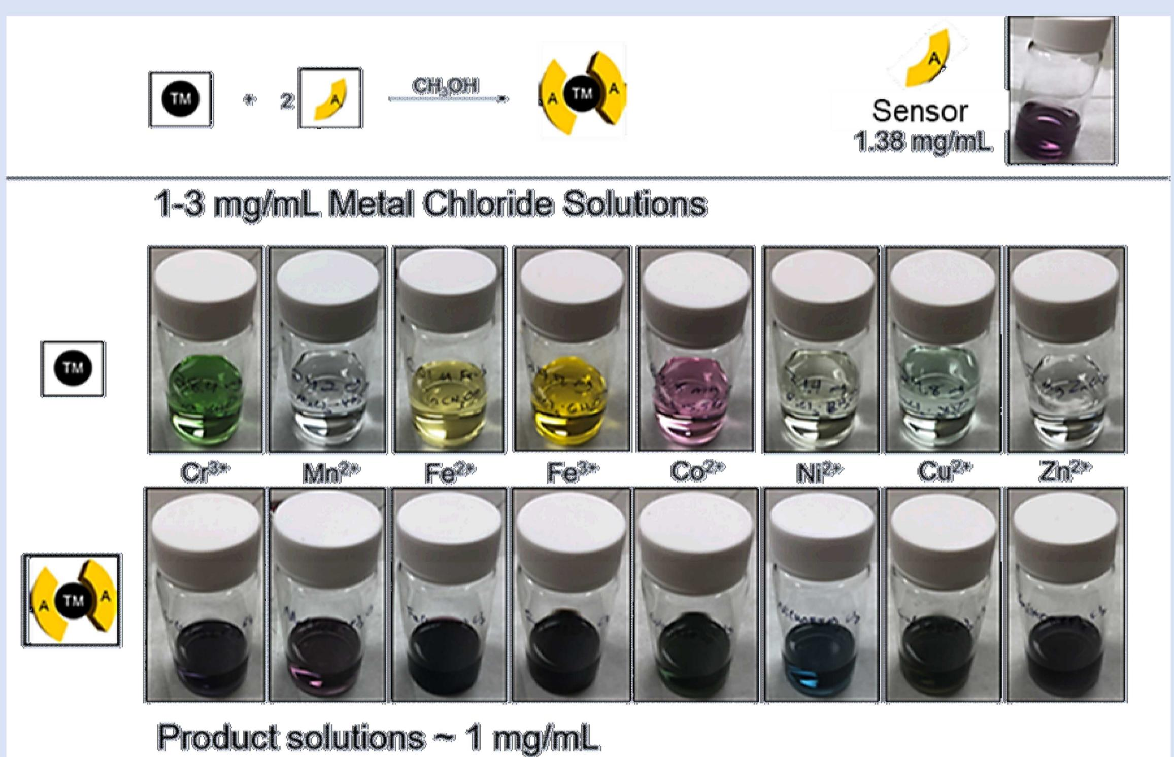
Colorimetric sensor mechanism using transition metal solutions (TM) with sensing organic molecule (A) to irreversibly form molecular (TM-2A) complex.
