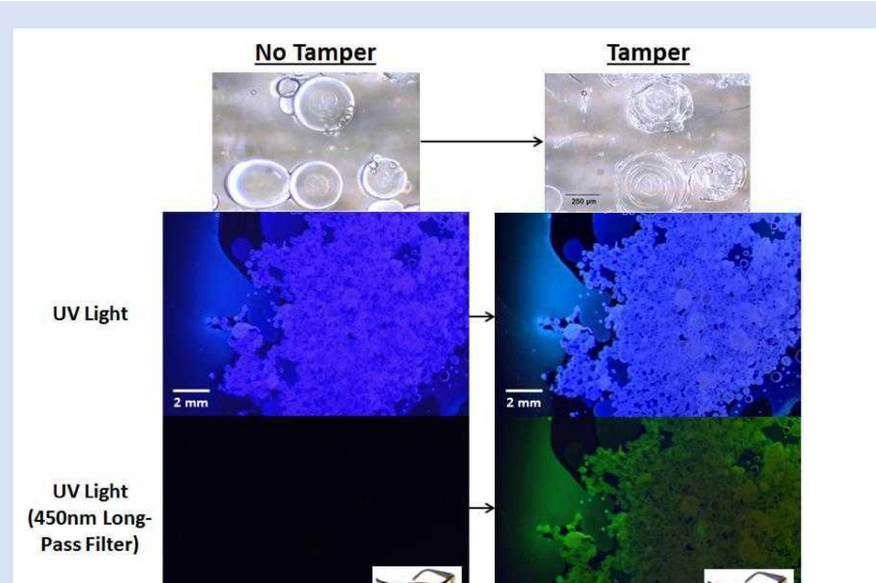
Summary of the tamper-indicating material concept. Pressure-induced microcapsule breakage is visualized by the presence of green luminescence when viewed through a long-pass optical filter (bottom-right image). An example of such a filter is the yellow-tinted sunglasses shown in the inset. No luminescence is evident in the undamaged system when viewed through the same filter (bottom-left image).
