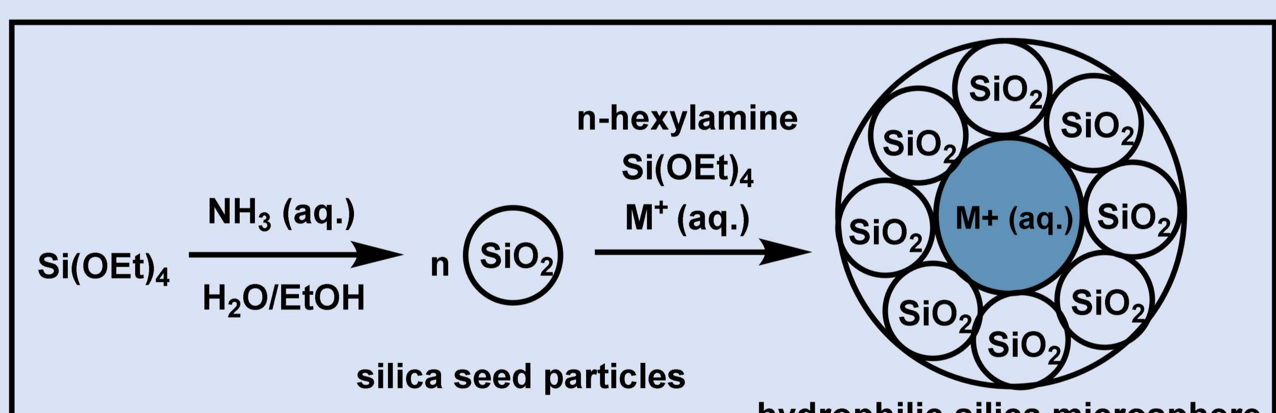
Strategy employed for hydrophilic silica microsphere synthesis. First, silica seed particles are created through the Stöber method; next the seed particles are assembled into a microsphere using an inverse Pickering emulsion; and finally, the sphere is solidified using additional Si(OEt)4.
