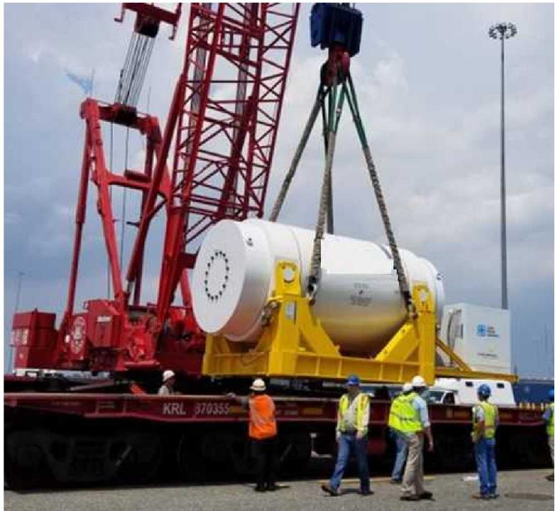
Photo of a SNF cask being moved from a container ship to heavy haul truck as part of a multi-modal, multi-jurisdictional international transportation test.
