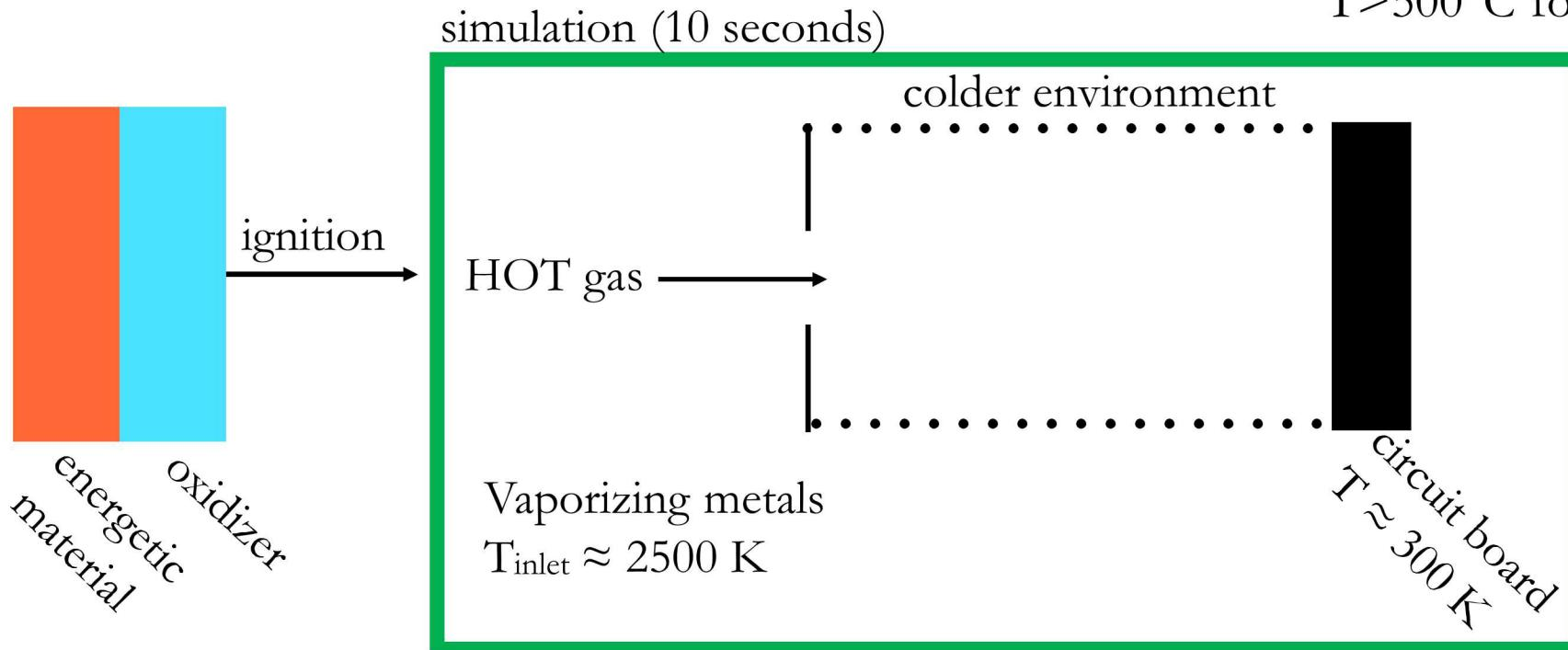
Hot gases entering colder environment -> condensation
