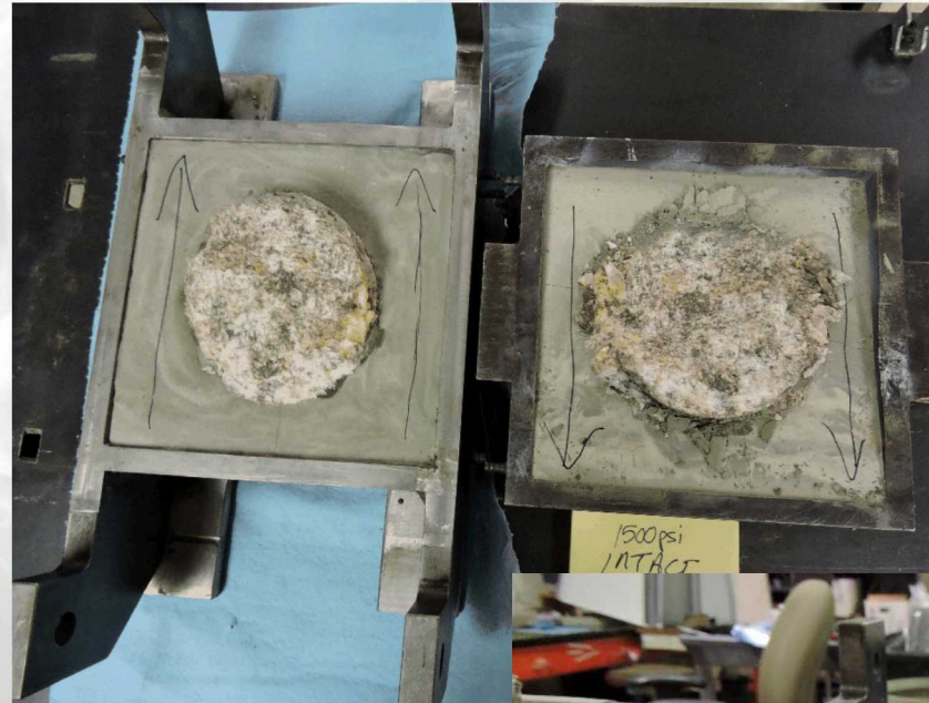
Intact test, \sigma_n = 1500 psi
