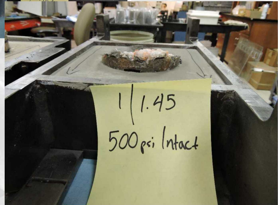
Intact test, \sigma_n = 500 psi, side view
