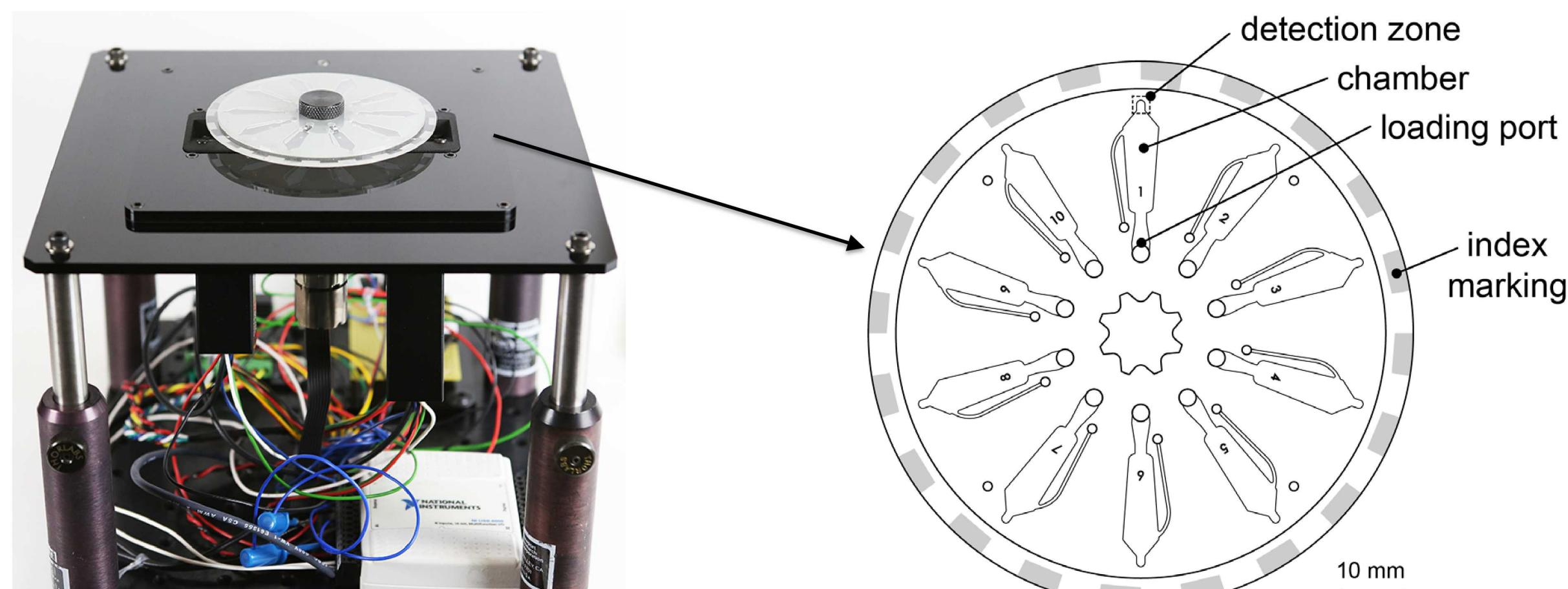
The microfluidic device at the heart of the platform is a simple three-layer disc designed to transport signal molecule-enriched microparticles from the center of the disc through a density matrix and into the detection zone located at the periphery of the disc. Cast acrylic sheets were ablated with a laser to form the structural top and bottom components held together by a pressure-sensitive adhesive layer into which the channels were cut.
