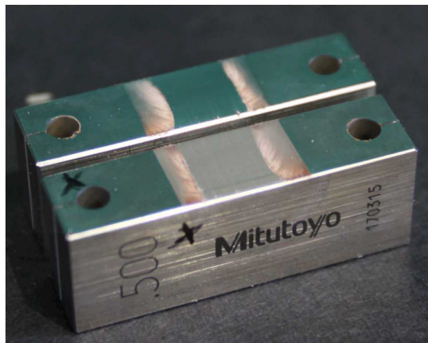
Fig. 5. Photo of gage block microchannel. The microchannel is cut into the block in the foreground. Particle deposition is evident along the side walls of the microchannel.
