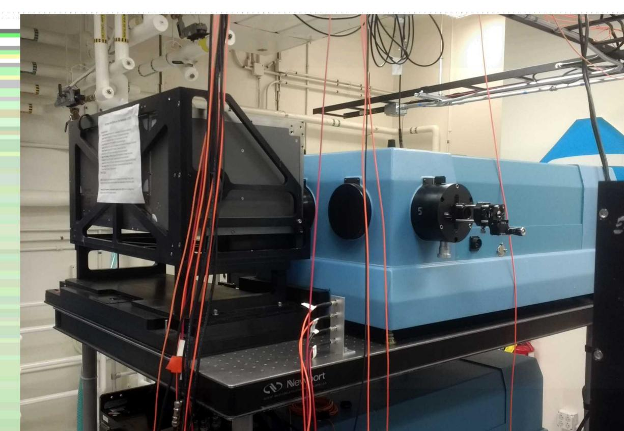
An absolutely calibrated streak spectrometer is lens coupled to a fiber optic cable which is used to image a 1-2 mm region on electrode surfaces on Z. Parameters of the streak spectrometers are:
