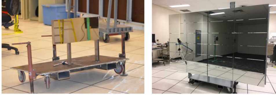
Figure 1. Single-facet test stand (left) and 24-facet lab-scale heliostat after initial alignment (right).
