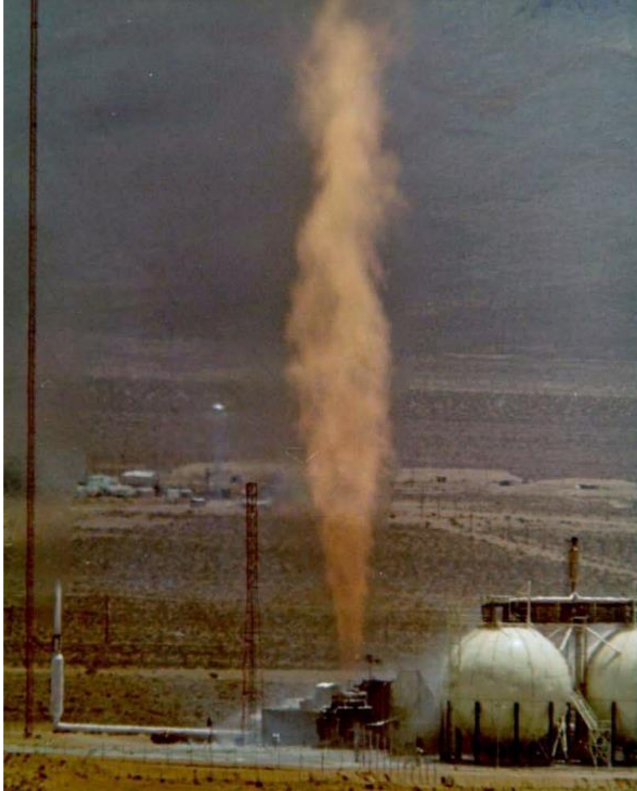
Figure 86. Test of the Phoebus 2A reactor at Test Cell C, June 28, 1968 (NASA). This southeast-facing image shows only the visible exhaust plume, but gives an indication of the radioactive plume released by each test. At the far left, excess hydrogen gas is being burned off at the Flare Stack (Los Alamos Scientific Laboratory).
