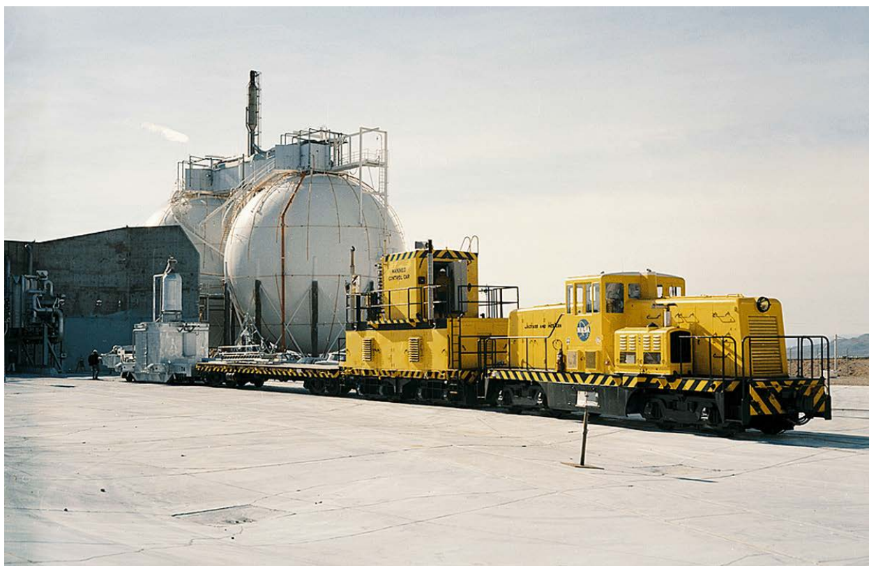
Figure 31. AR-11 (25-3210), Railroad Transport System delivering the PEWEE nuclear test vehicle to the Reactor Pad (RSL, 1967).
