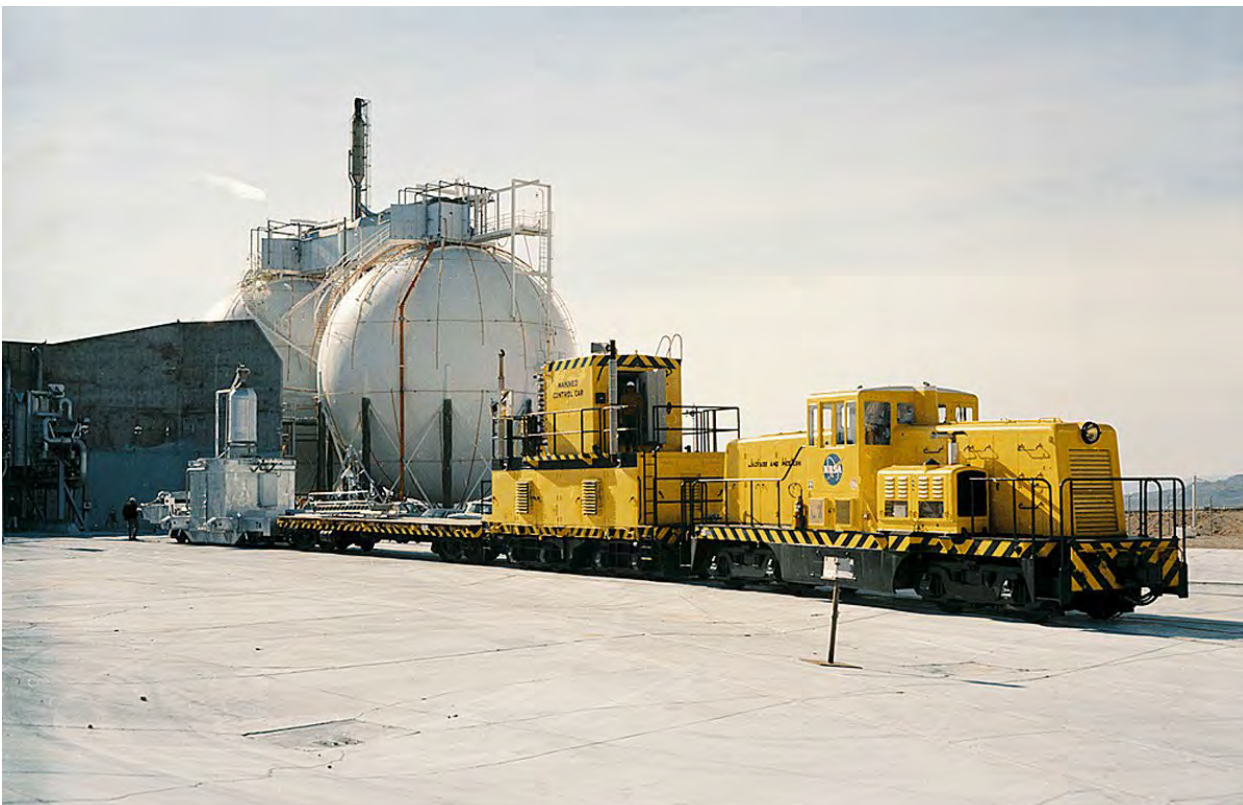
AR-11, Railroad Transport System delivering the PEWEE nuclear test vehicle to the Reactor Pad (Photo Source: RSL, 1967).
