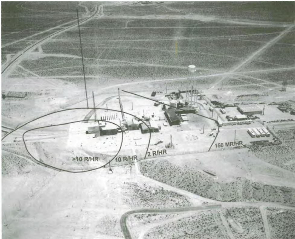
Test Cell C overview facing east-southeast. This image shows radiation levels following the June 25, 1965 Phoebe 1A reactor core ejection incident. It was taken immediately before the major 1965-1966 upgrade and includes full images of both towers (Los Alamos, reproduced from Dewar 2004:129, 1965).
