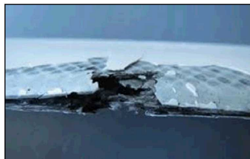
Trailing Edge Disbond and Fracture Damage
