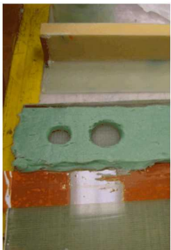
Voids in bond joint
