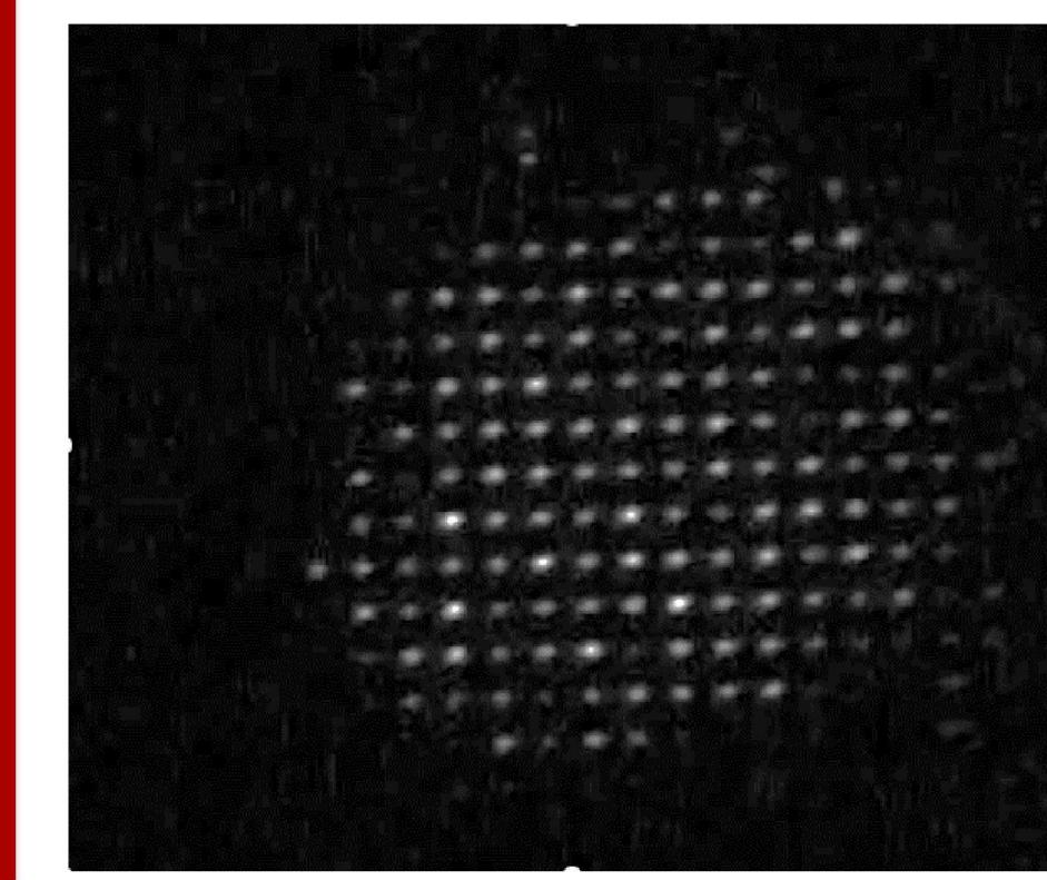
**Top Down View of Vertical GaAs PCSS device with parallel current filaments (higher current, longer lifetime)**
