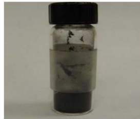
Isolation of kerogen from Mancos shale
