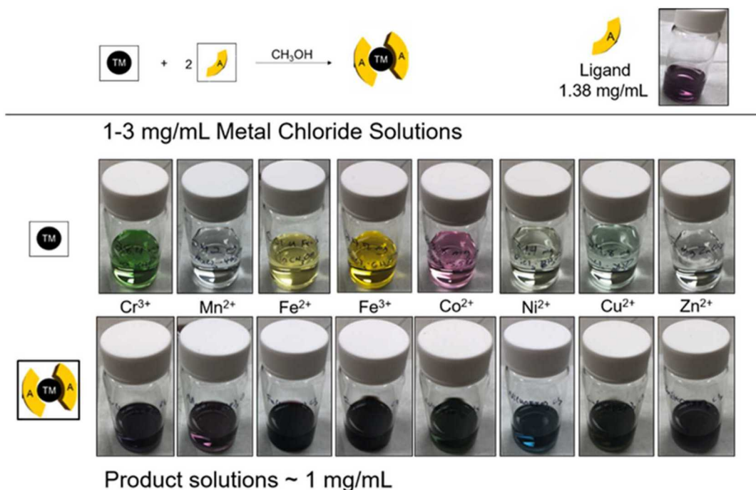
FIG. 1. Colorimetric sensor mechanism using 3d transition metal solutions (TM) with sensing organic molecule (A) to irreversibly form molecular (TM-2A) complex.
