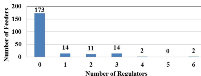
Figure 1. Histogram of the number of voltage regulators on each feeder.
