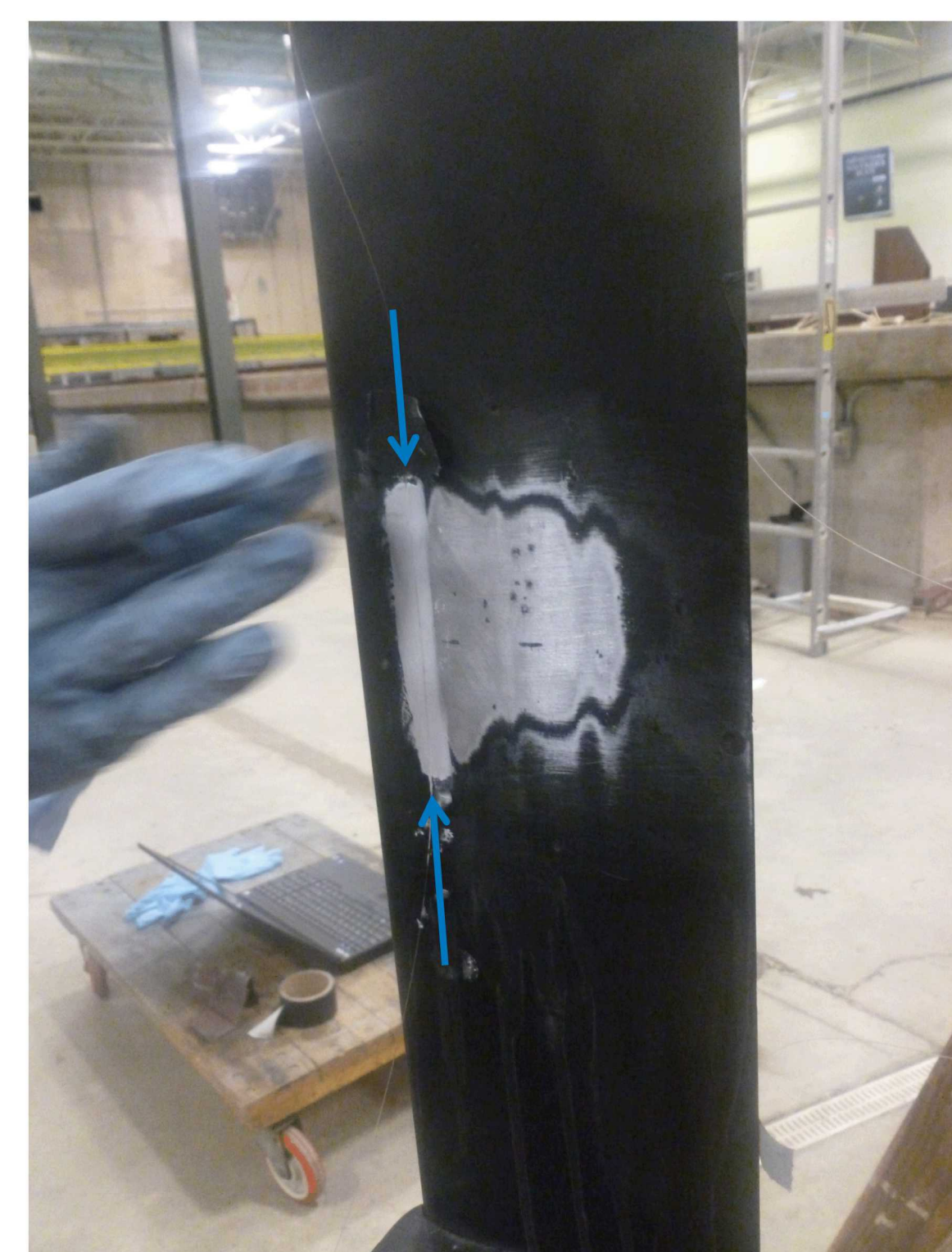
The bare os 3200 FBG sensor used for testing
