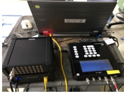
Fig. 4. The electronics for data collection and signal processing are shown with the ALMM (left) and the JSR-15 (right).
