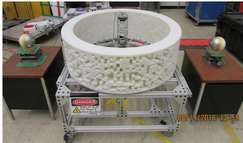
Figure 4 - CONFIDANTE with two LLNL PuO 2 hemispheres facing the central detector. Each hemisphere was coupled to a solid HDPE hemisphere on their backsides.
