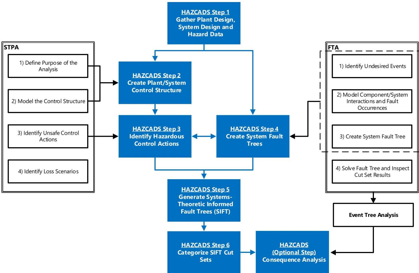
Utilization of fault trees allows event trees to be used for consequence analysis (i.e., assessing the impact of digital components on core damage states).
