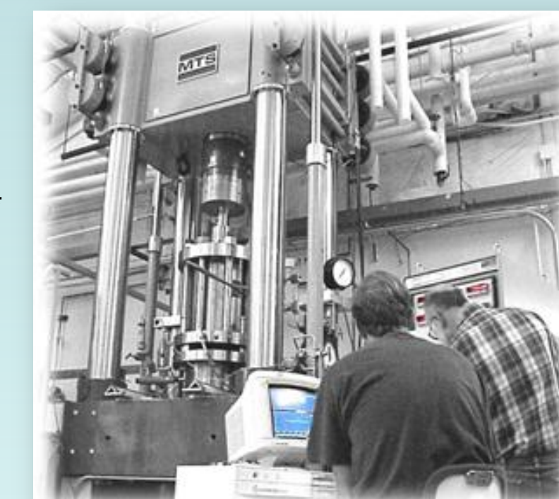
Geomechanical testing for acoustic and ultrasonic imaging of rock deformation
