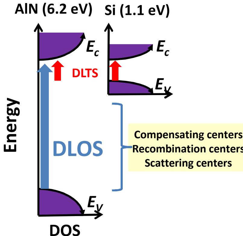
**Solution: Deep Level Optical Spectroscopy (DLOS)**
