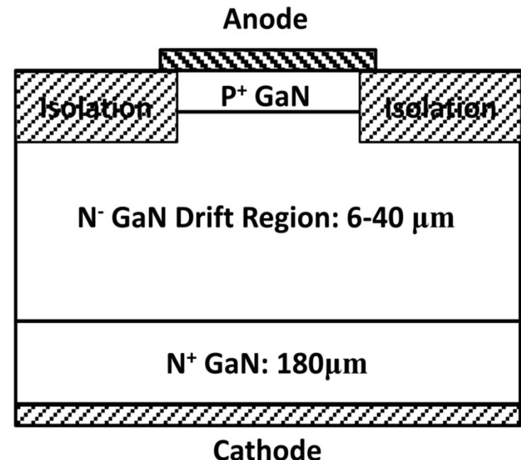
Vertical devices have smaller area per device, higher device yield, increased breakdown voltage, and larger current drive in comparison to lateral device structures.
