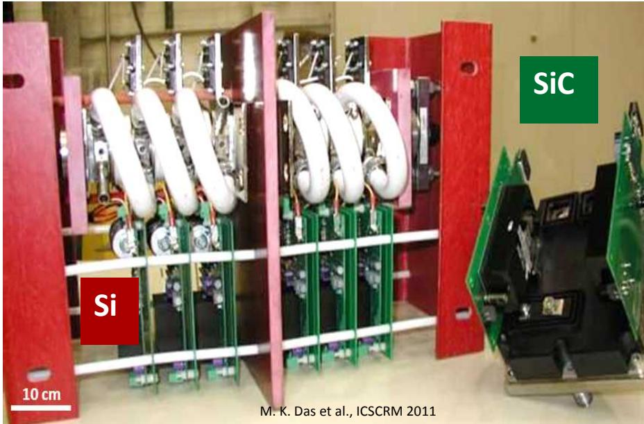
SiC is 10% the volume and weight of Si for equivalent capability (10 kV, 100 A)
