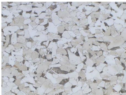
Figure 3. Optical microscope images of polished and etched cross section of the lid of the second Li pre-heater.
