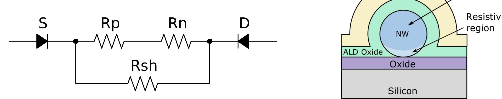
Resistance of the n- and p- sections of nanowire can be estimated from their charge density at a given gate voltage:
