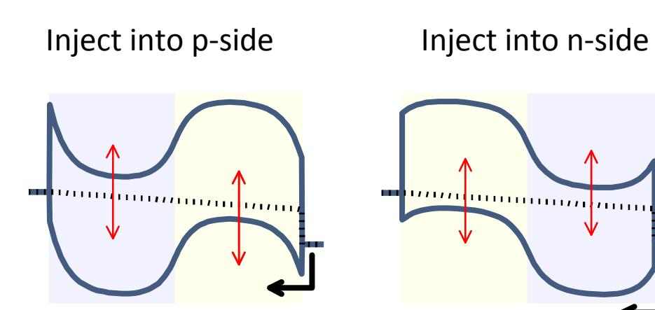
These band diagrams also reveal why the current saturates when sweeping the opposite gate voltage. Current becomes limited by the injection from the contact, so the opposite gate cannot increase the current any further. Both gates need to be enabled to get significant current levels.
