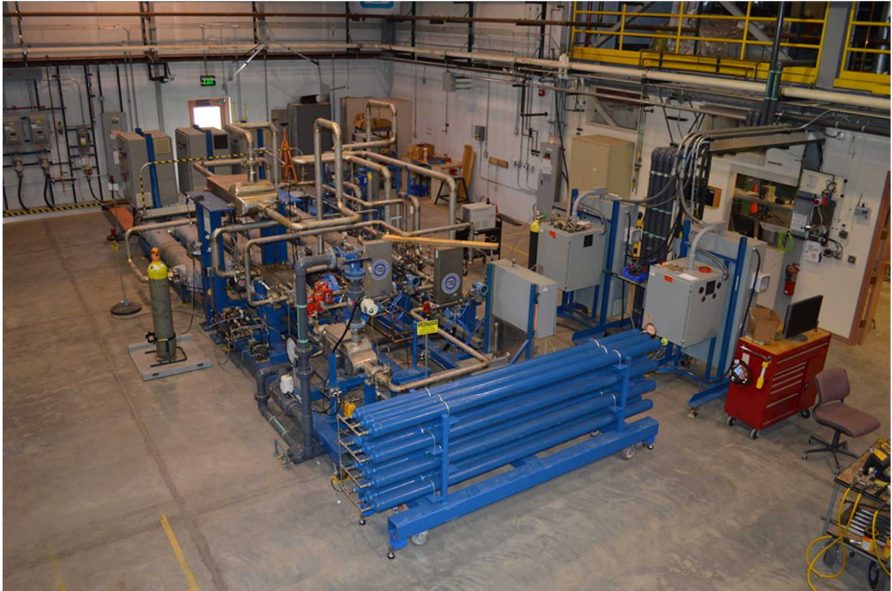
Figure 3: Sandia National Laboratories recompression closed Brayton cycle testing platform.
