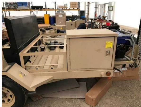
Storage box and backup generator mounted to AMF3 trailer.
