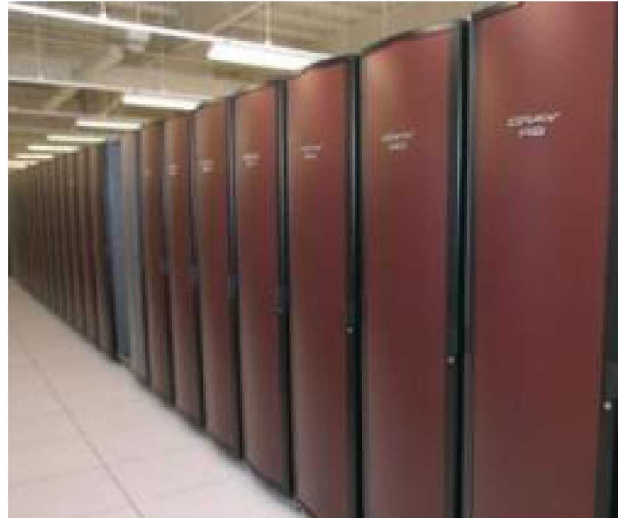
Figure 1: Sandia's Red Storm is approximately 3,500 sq. ft. and uses 2.2 megawatts.
