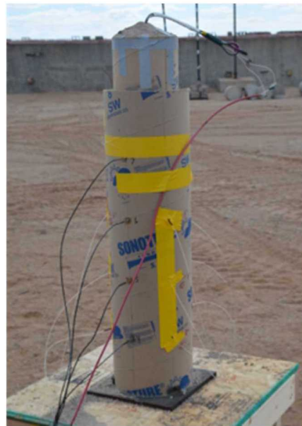
Fig. 3. Experimental charge with FLRS, timing pins, and continuous velocity probes installed.
