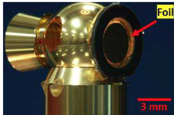
Sample on hohlraum w/ Be tamper attached
