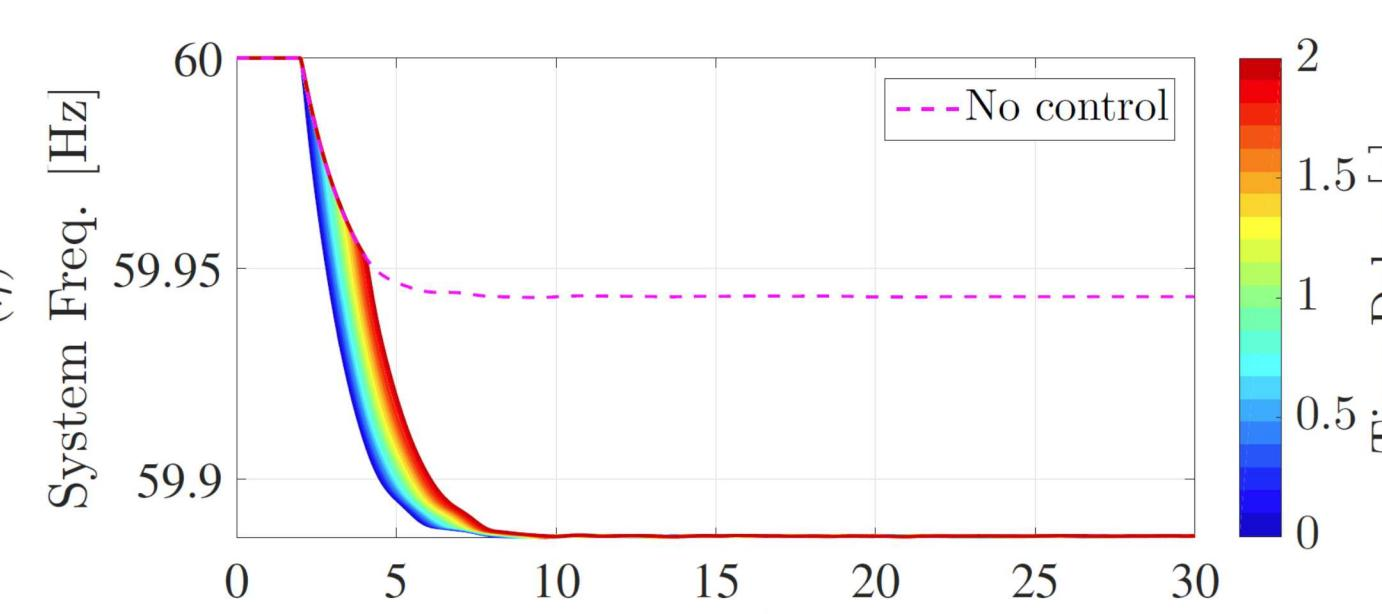
Freq. response when  $\eta = -1$  for different delays in the control action
